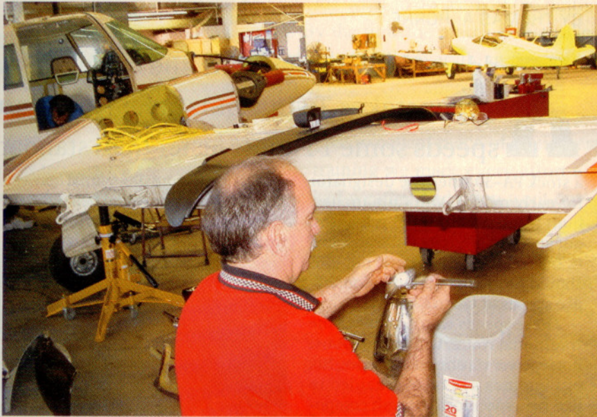
Ailerons, flaps, and stabilator have been sent to Williams Airmotive for reskinning, and LoPresti mechanics prepare to install speed mods (above). Fuel lines for the J.L. Osborne tip tanks are routed to the fuel selectors (left), while four new fuel cells from Eagle Fuel Cells (above right) await installation.
