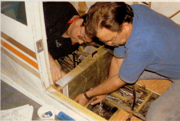
Ailerons, flaps, and stabilator have been sent to Williams Airmotive for reskinning, and LoPresti mechanics prepare to install speed mods (above). Fuel lines for the J.L. Osborne tip tanks are routed to the fuel selectors (left), while four new fuel cells from Eagle Fuel Cells (above right) await installation.
